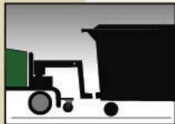
Insert tube on the front of the WasteCaddy attaches to the bottom of the dumpster.
