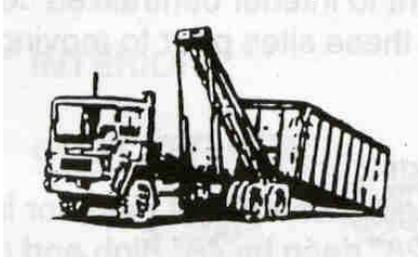
Figure 5. Truck Delivering Roll-Off Container.
