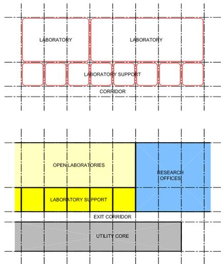
The above description of the planning module also includes the organized and systematic delivery of laboratory piped services, HVAC, fume hood exhaust ducts, power and signal cables. If these services are delivered to each laboratory unit in a consistent manner, then changes in laboratory use requiring addition or deletion of services will be easy to accomplish because of the constant nature of the infrastructure.
