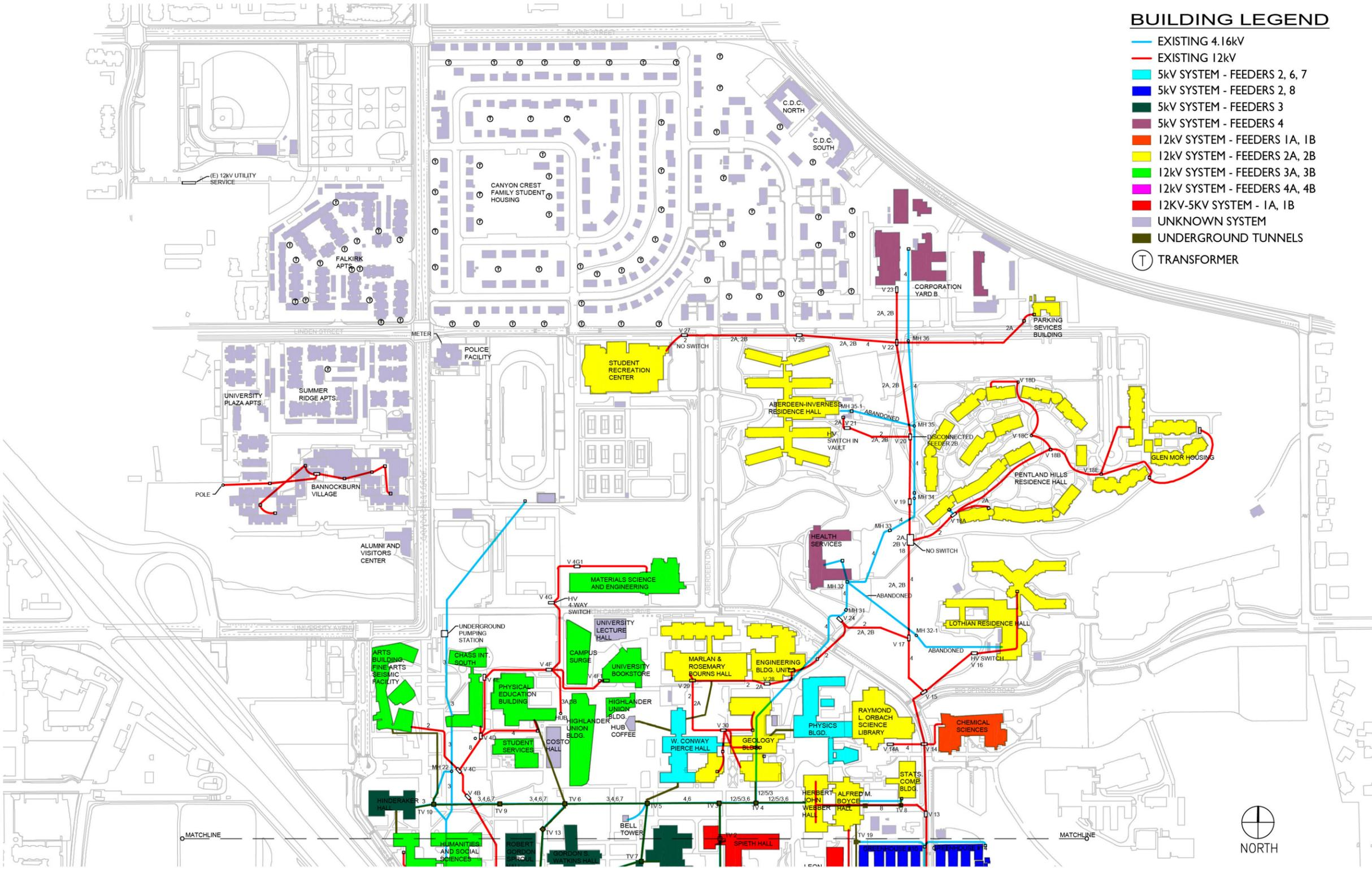
Figure 2.3—Existing 4.16kV and 12kV Electrical Site Plan by System and Feeder—North
