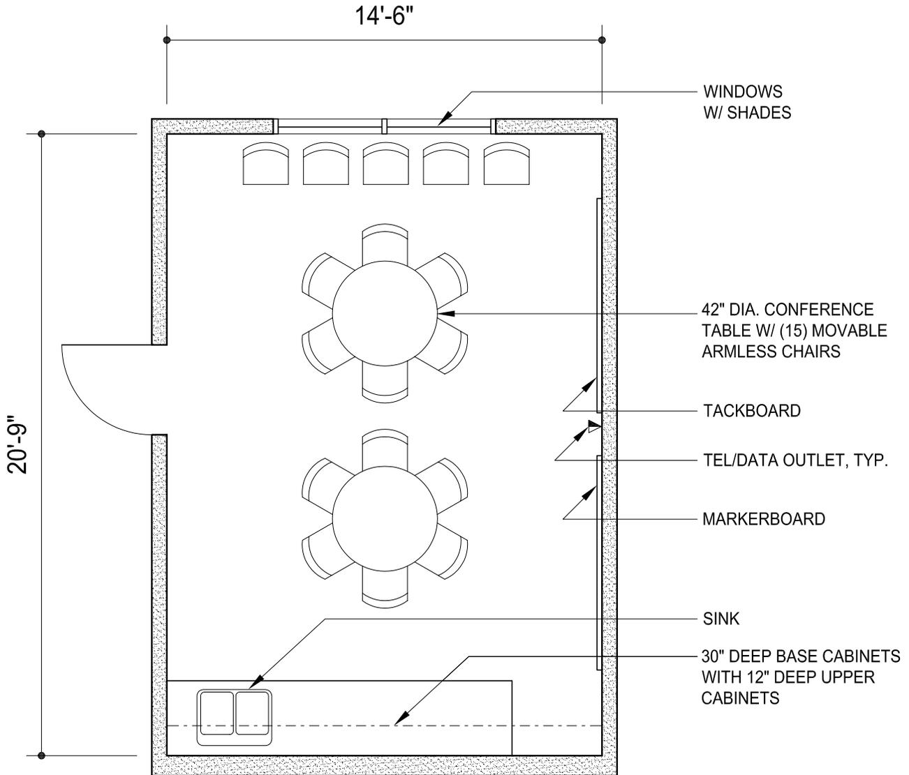
**A1.0****DETAILED SPACE REQUIREMENTS AND DIAGRAMS****NOTE: DIAGRAMS ARE FOR REFERENCE ONLY**
