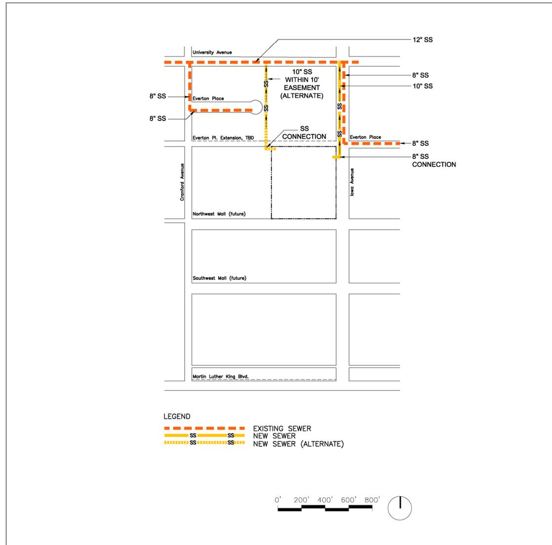
Figure 5.2.2-1: Sanitary Sewer System Diagram
