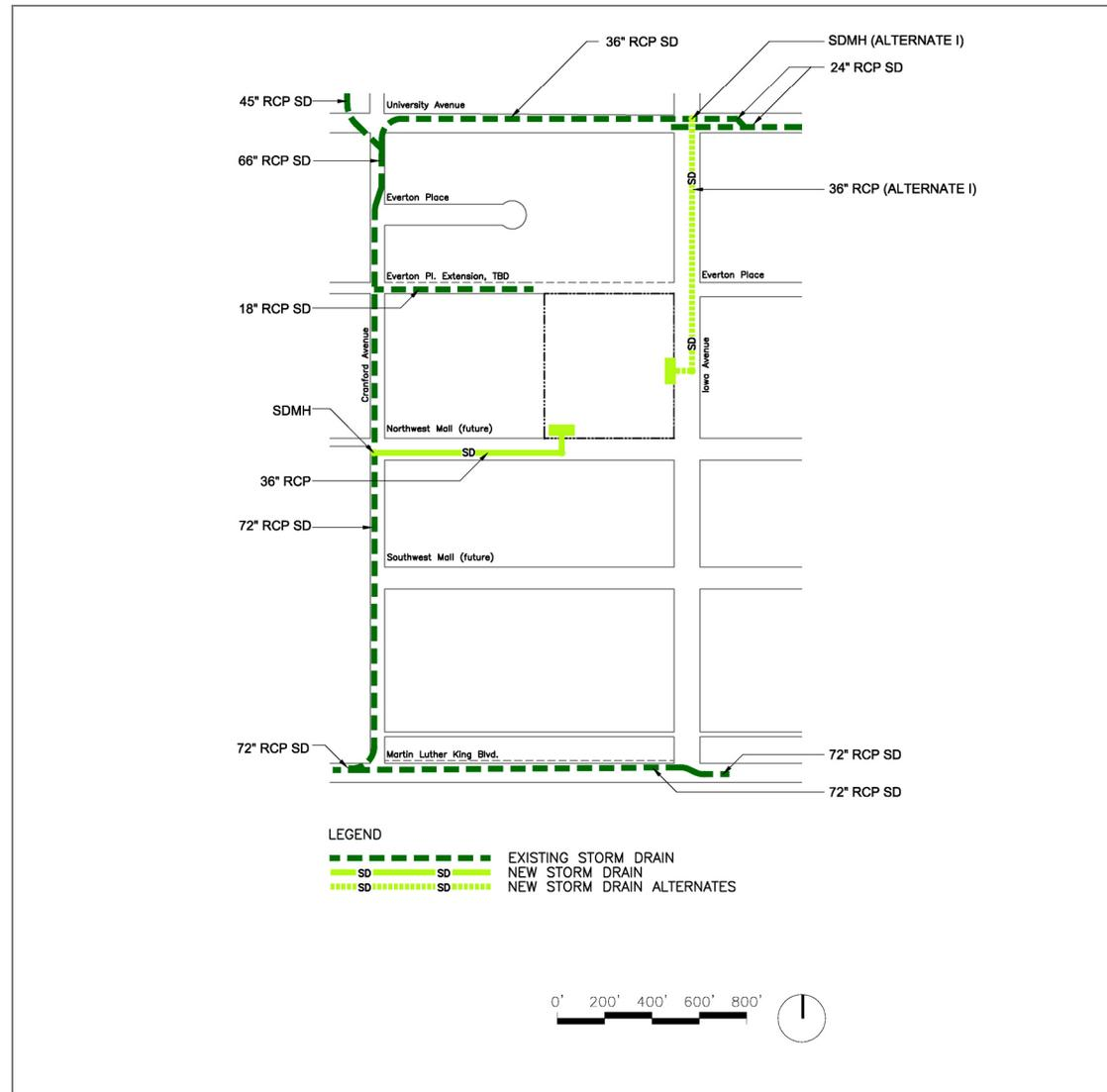
Figure 5.2.3-1: Storm Drainage System Diagram
