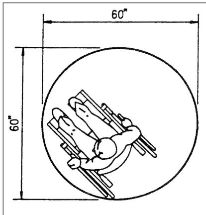
**Figure 3.5-1: 60-Inch Diameter Space Diagram**
