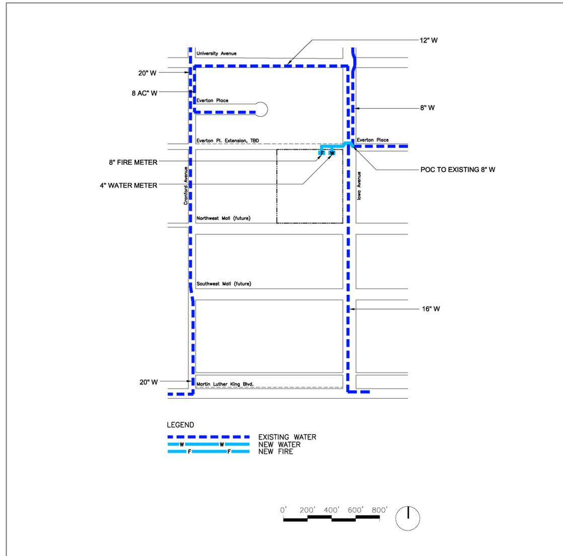
Figure 5.2.1-1: Water and Fire Protection Diagram
