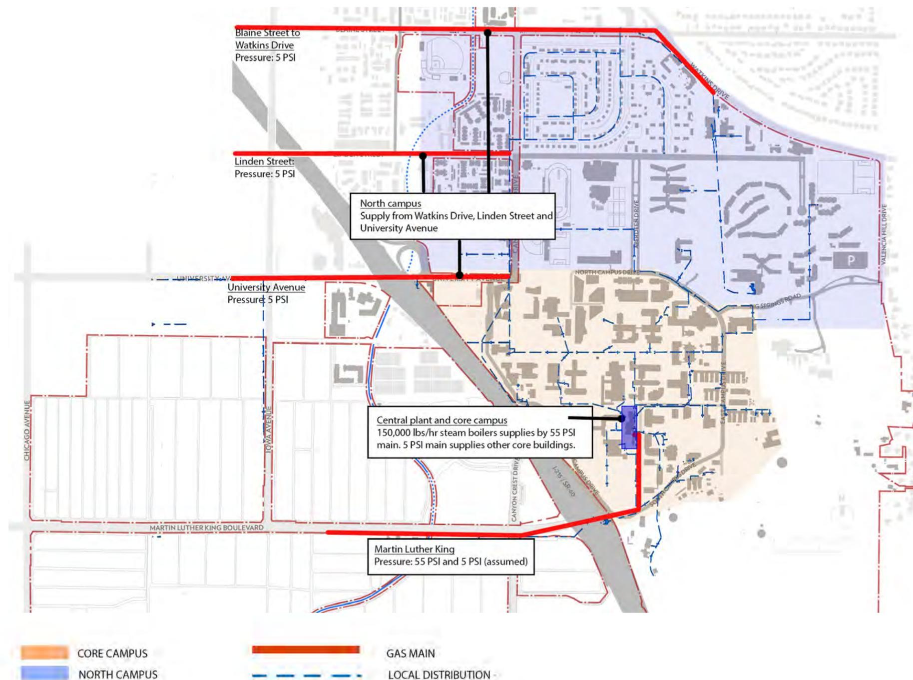
This figure is a diagrammatic representation of an infrastructure network that is based available drawings and in person conversations with UCR personnel. They are representative and likely to have some inaccuracies.
