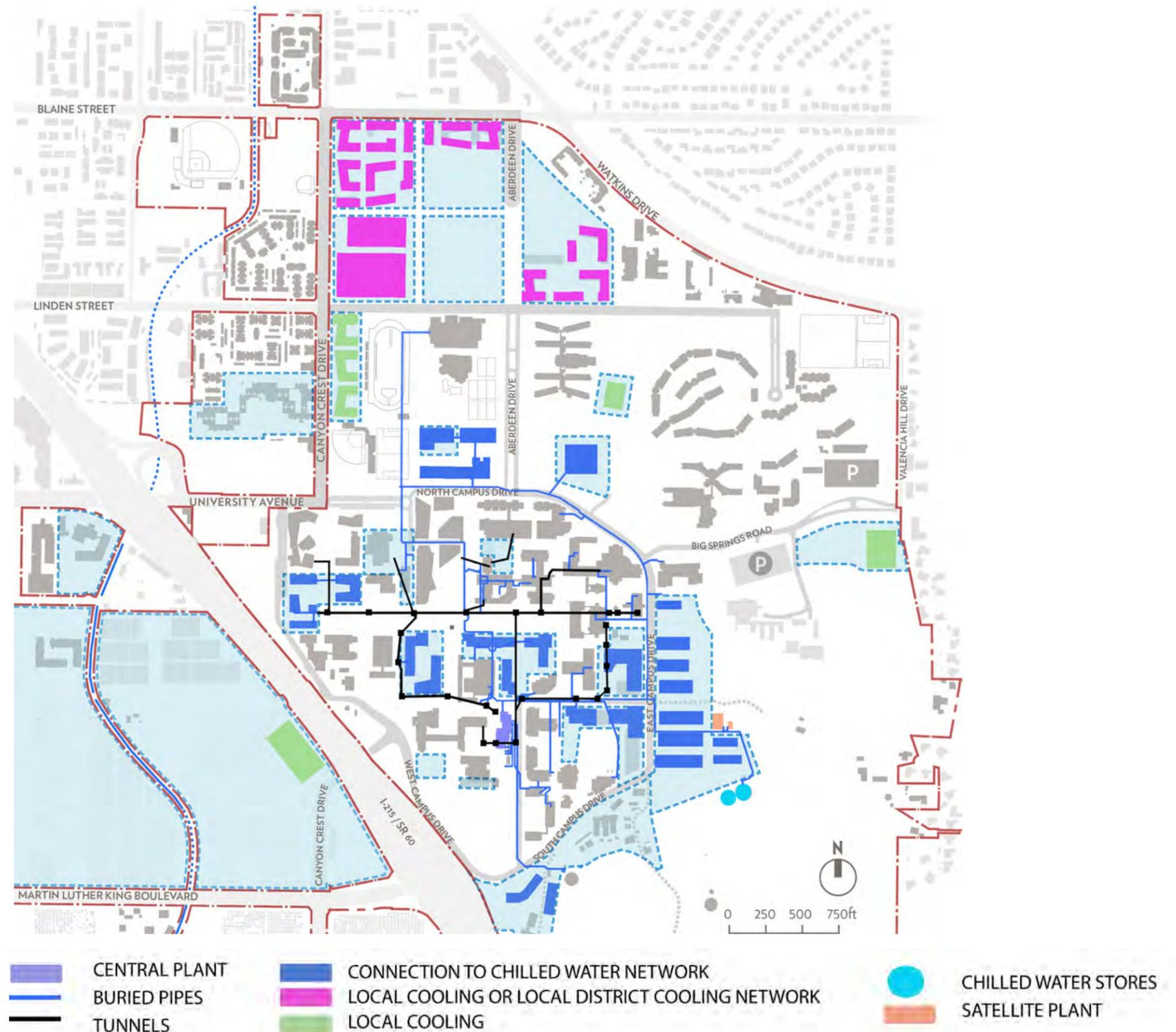
This figure is a diagrammatic representation of an infrastructure network that is based available drawings and in person conversations with UCR personnel. They are representative and likely to have some inaccuracies.
