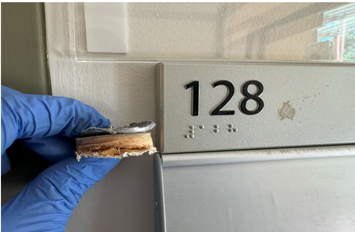
Photograph 18: Lead shielding, behind wood panels in room 128.
